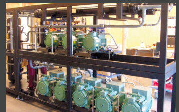
All LILLNORD units are delivered with a BITZER compressor to safeguard operational reliability
